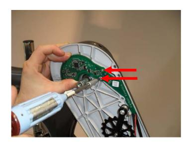
6.4. Align the Main Junction Board PCB Board flush against the Cleandrive and reinstall the securing screws as demonstrated.
