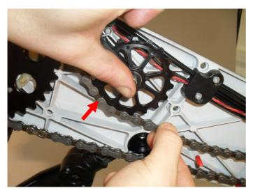
7.3. Continue to apply upward pressure to the Chain Tensioner in order to refit the chain to the Chain Tensioner sprocket as shown.
