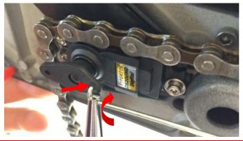
5.7. It helps to rotate the spring away from the Servo to line up the end of it with the hole in the Servo Horn.
