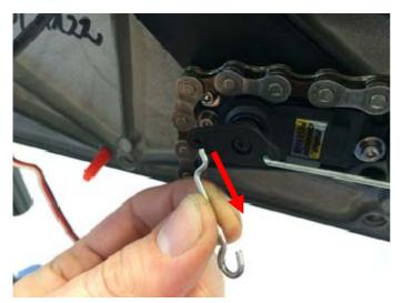
4.13. Remove the E-Shift Balance Spring from the servo by unhooking from the E Shift Spring Balance Link, then remove the E-Shift Spring Balance Link from the servo.
