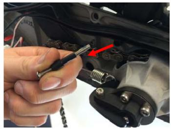
4.15. Use a 2.5mm Allen key and take care to keep the E-Shift Spring Spacer with the bolt.
