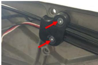
4.7. Remove the Cable Guide Upper by unscrewing the two retaining bolts using a Torx T15
