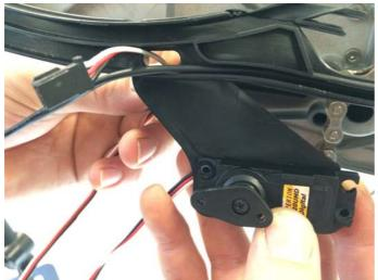
5.2. Front view of the Servo correctly mounted into the Cable Guide Lower.
