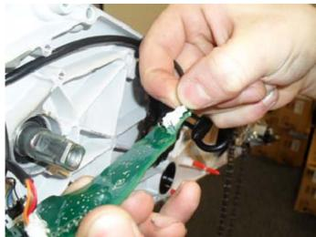
4.4. Hold the edge of the Main Junction Board PCB as shown, and remove the 2 pin white connector. This is the Rear Sensor.
