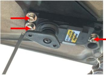
5.5. Secure the Servo in position with the three M3 x 25 Caphead bolts, ensuring the washers are present.
