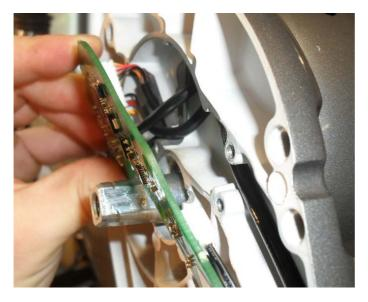
6.3. Begin to close the Main Junction Board PCB against the Cleandrive<sup>®</sup>. This photo demonstrates the correct cable routing. Ensure that no cables get pinched or trapped.
