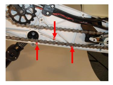
8.1. Ensure the three Chain Pins are installed correctly and that the chain runs through them as shown.
