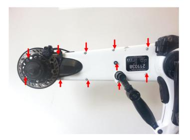
2.1. Using a T25 Torx Bit, unscrew the eleven Magform Bolts (11) as shown.
