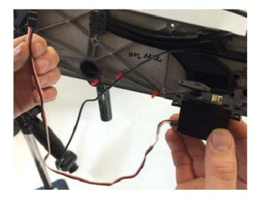
4.22. Completely remove the Servo as shown.
