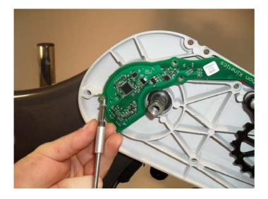
4.2. Remove the Junction Board by undoing the retaining bolts.
