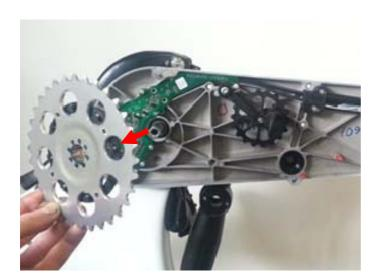
3.3. Allow the Chain to hang free and remove the Chainring from the Bottom Bracket Spindle as shown.
