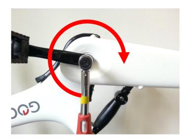
10.4. Now install the Right-Hand Crank Arm Bolt and tighten with a wrench to a 35-40Nm torque.
