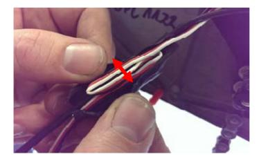
4.11. When the shrink wrap has been removed, there may be excess wiring coiled up underneath.
