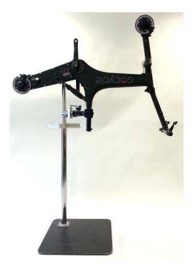
1.1. Invert the G2 and locate in a work stand. Remove both PitStopWheels®.
