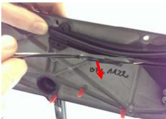
4.9. Pull the wires out of the Cable Guide Lower to reveal the heat-shrink-wrapped section. These wires are the Servo Controller Cable (with the flat black connector) and the Rear Sensor Cable (with the white connector).
