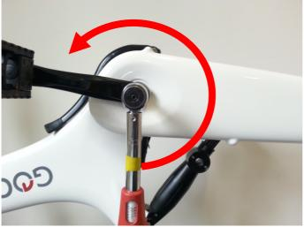
1.2. Use a wrench with an 8mm Hex bit to undo the Right-Hand Crank Arm Bolt (2283).
