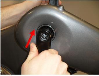
10.3. Align the Right-Hand Crank Arm to the Bottom Bracket spindle and then slowly rotate to help locate the Dowel Pins in the Chainring.
