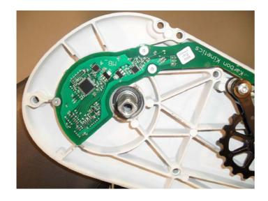
4.1. Once the Chainring has been removed, the Main Junction Board (JB) will be v as shown.
