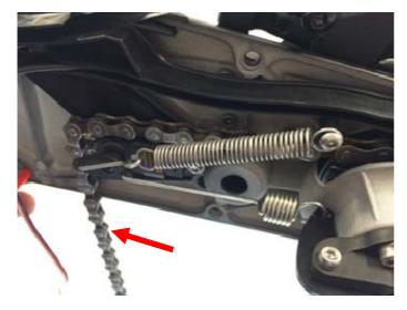
4.6. Allow the chain to rest as shown so that both balance springs are free and accessible.
