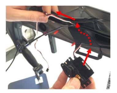
5.1. To fit the new Servo, first loop the Servo Controller Cable through the large lower hole in the Cable Guide Lower, then back up through the smaller upper hole. Whilst pulling the wire through, fit the servo back into its mounting hole.
