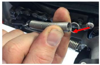
4.12. Unhook the E Shift Balance Spring from its mount on the Cleandrive.
