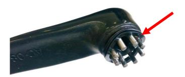
1.4. Take care when removing the crank arm and ensure to keep all 8 dowel pins (2175) located as well as all 4 Carbon Steel Wave Springs (2225).
