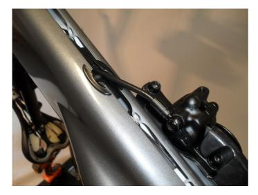
9.1. Align the Cleandrive® cover ready for reassembly.
