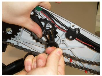
7.2. Apply light upward pressure to the Chain Tensioner in order to remove the Lockshock® pin.
