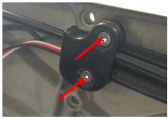
5.19. Install both Cable Guide Upper bolts using a Torx T15 or Philips screwdriver depending on Gocycle Frame Number.
