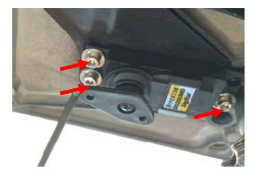
4.19. Remove the three M3 x 25 Caphead Servo retaining bolts using a 2.5mm Allen Key. Make sure to keep the washers for reinstallation.
