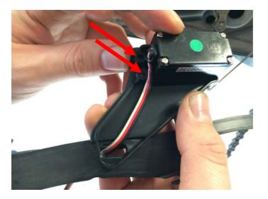
5.3. Rear view of the Servo correctly mounted into the Cable Guide Lower. Take care to ensure the Servo Controller Cable clears both of the bolt holes.
