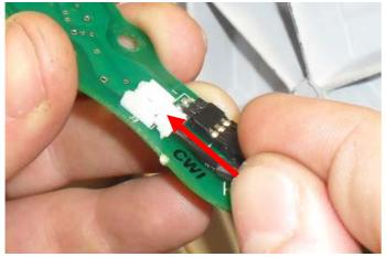
6.2. Connect the Rear Sensor Cable and ensure it is fully closed.
