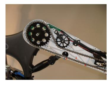
8.3. Check that the Chain is fitted to the Chainring and the Chain Tensioner sprocket correctly as shown.
