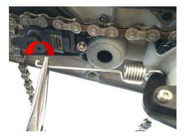
4.17. Unhook the Servo end first. Using pliers, rotate the E-Shift Spring towards you so that the hooked end becomes free of the Servo Horn, then pull away from the Servo.
