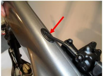
9.2. Take care to line up the brake hose seal correctly, as shown.
