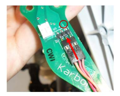
6.1. Reconnect the Servo Cable. Ensure that the brown cable aligns with the negative pin.
