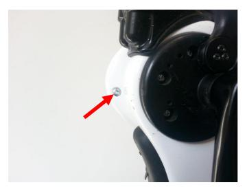
2.3. Unscrew and remove the remaining Magform Bolt (11).
