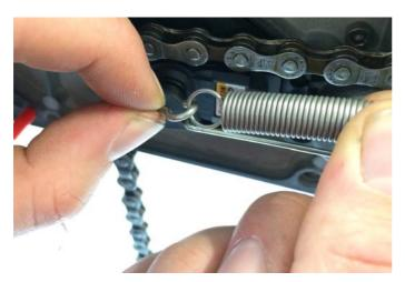
5.10. Connect the end of the E-Shift Balance Spring to the E-Shift Balance Spring Link as shown.
