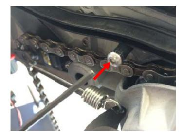
4.14. With the E-Shift Balance Spring removed, the retaining bolt can also be removed.
