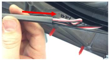
5.15. Cover both the Servo Cable and Rear Sensor Cable with the shrink-wrap, ensuring all of the folded wiring is covered.
