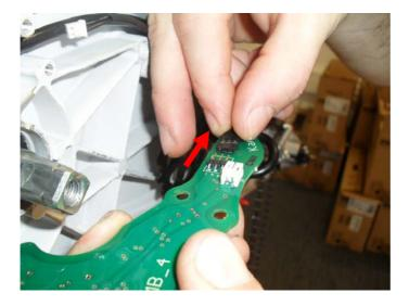
4.5. Remove the 3 pin connector as shown. This is the Servo Cable.
