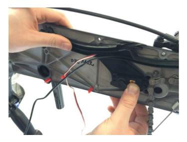
5.4. Reattach the Cable Guide Lower with Servo to the Cleandrive.
