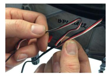
5.14. Check the length of the new Servo Controller Cable by running it up through the Cable Guide Lower so that the connector block is near its mounting location on the Main Junction Board.
