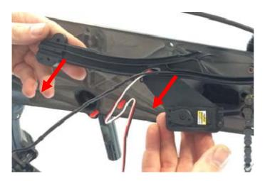
4.20. Remove the Cable Guide Lower along with the Servo from the Cleandrive by pulling it away.
