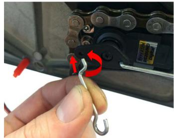
5.9. Locate the E-Shift Balance Spring Link into the Servo Horn as shown.
