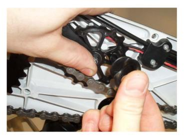
Note: You do not need to completely remove the chain. Derailing it from the Chain Tensioner and Chainring will be sufficient for access to the servo.
