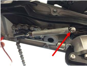
5.12. Hook the hooped end of the E-Shift Balance Spring on to the bolt as shown.
