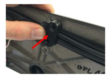
5.18. Insert the Rear Brake Hose and the combination of Servo and Rear Sensor Cable in to the Cable Guide Lower channels and mount the Cable Guide Upper to secure them in place by hand as shown.
