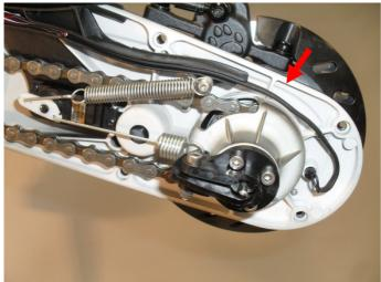
8.2. Check the Servo Balance Springs are installed correctly as shown.
