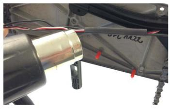
5.17. Use a Heat Gun to tighten the shrink-wrap around the Servo Cable and Rear Sensor Cable.
