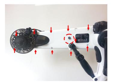
9.3. Install the 11 Magform Bolts back into the Cleandrive® noting the position of the fender guide bracket.
