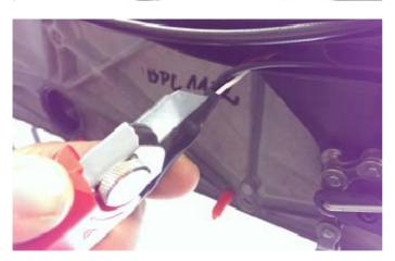
4.10. Use a sharp blade to very carefully cut off the shrink-wrap, taking care not to damage the wires underneath.
