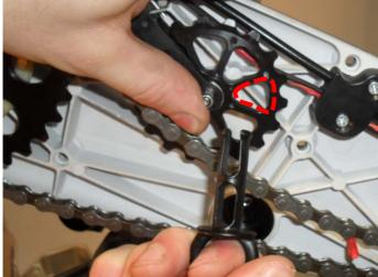
3.2. Release the Chain from the Chain Tensioner and use the LockShock<sup>®</sup> Pin to secure the Chain Tensioner as demonstrated.
