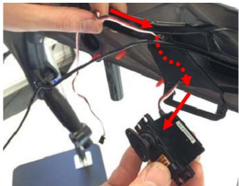
4.21. Remove the Servo from the Cable Guide Lower. This is done by pulling the Servo out of the Cable Guide Lower and threading the cable out.
