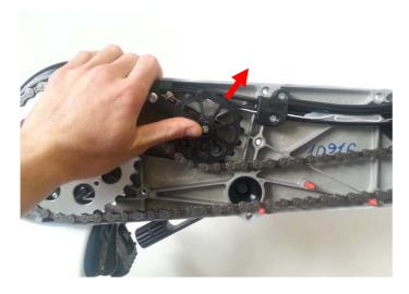
3.1. Use your thumb to apply upward pressure on the Chain Tensioner as shown.
