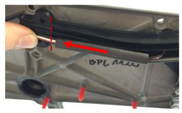
5.16. Insert the cable in to the Cable Guide Lower and check that the shrink-wrap does not extend under the Cable Guide Upper as shown.
