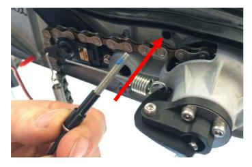
5.11. Install the E-Shift Balance Spring retaining bolt along with E-Shift Spring Spacer using a 2.5mm Allen Key.
