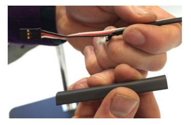
5.13. Replace the Servo cable shrink-wrap. Cut a 50mm length of 8mm shrink-wrap.
