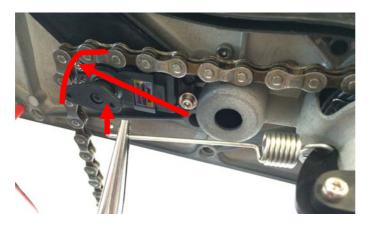
5.6. The Chain must now be looped back over the Servo before the Servo springs can be reinstalled.
