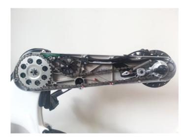
2.4. The Cleandrive® Cover can now be removed ready for internal inspection.
