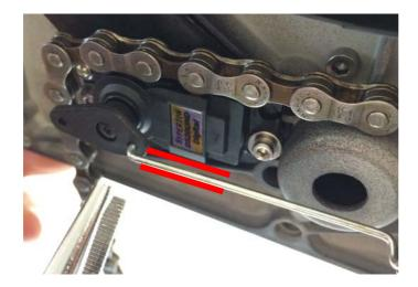
5.8. This shows the E-Shift Spring correctly installed.
