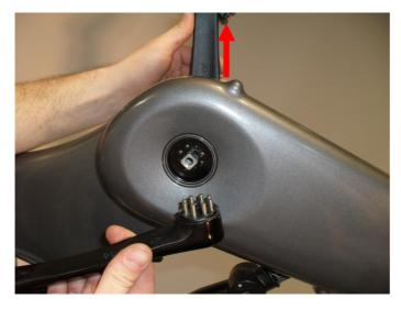
10.2. Hold the Left-Hand Crank Arm vertical as shown and have the Right-Hand Crank Arm ready to install.
