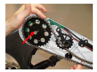
7.1. Re-install the Chainring on to the Bottom Bracket Spindle and locate the Chain on to the Chainring as shown.
