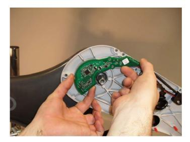
4.3. Remove the Main Junction Board PCB taking care not to touch the components on the board, as shown.
