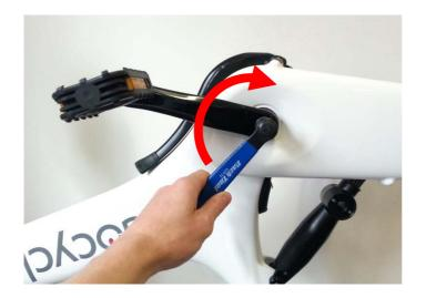
1.3. Use a square taper crank puller to remove the Right-Hand Crank Arm (2061).
